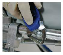
Fig 2 Position Quick Release Clip
