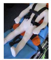
Fig 7: Shoulder straps in place for crotch strap buckle
