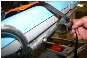
Fig 2: Position the U bracket onto the side of the backrest frame
