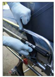
7. Fit the two large metal clips from the large restraint to the moulded sides at the rear of the outer shell and push up to lock tight.
