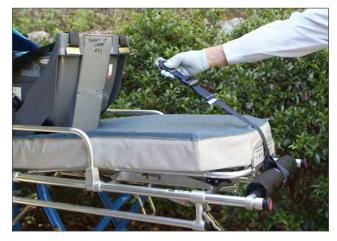
10. Attach the baby capsule tether strap to the standard baby capsule strap and tighten.
