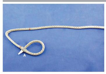
**Step #2** – Attach the end to a fid and pass them through the center of rope at Mark A.
