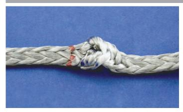
**Step #4** - Pull end hard to roll "inside-out" at Mark A.
