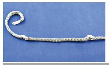
**Step #7** – Pull tight to roll the knot "inside-out" at Mark B.
