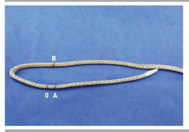
A "Locked Brummell Splice" may be made, using only one end of the rope, in most Hollow Braid ropes.
