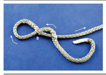
**Step #11** - Pull short end up -while pulling the standing end down as shown.
