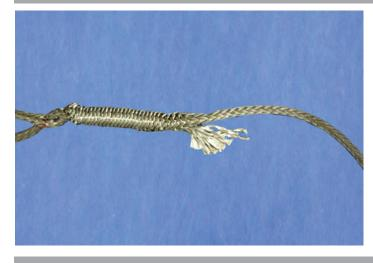
**Step #14** – Remove fid and tape, pull End 1 until 1/2 of a full fid length is exposed at the exit point. Fan all the ends out and cut ends on an angle to provide a smooth taper.
