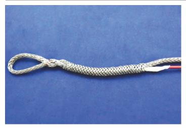
**Step #13** – Finally, bury tail into standing end. Attached the fid to the tail of the rope. On the standing part of the rope, measure one rope diameter below where the tail exits the standing part of the rope, this will be the entry point.
