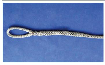
**Step #15** – Once the taper is complete, milk the rope back from the eye towards the exit point, this should bury the tapered tail back into the rope.
