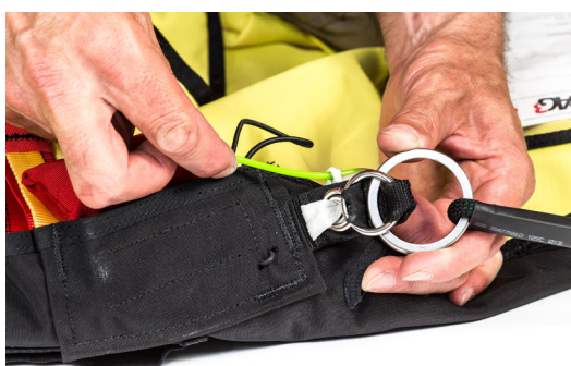
Figure 46 – Placing the green string in the loop
