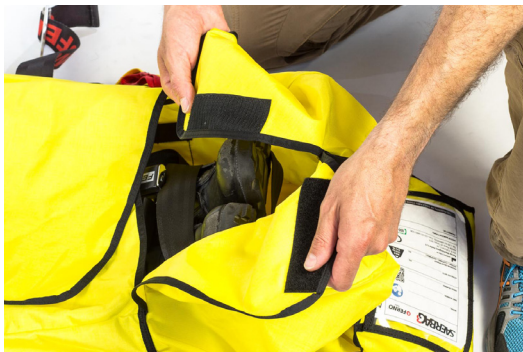
Figure 21 - Closing the foot area
