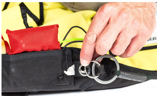
Figure 44 – Flipping the small ring over the large one
