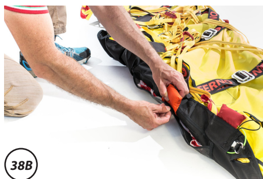
Figure 38 - Securing the handle to the Velcro
