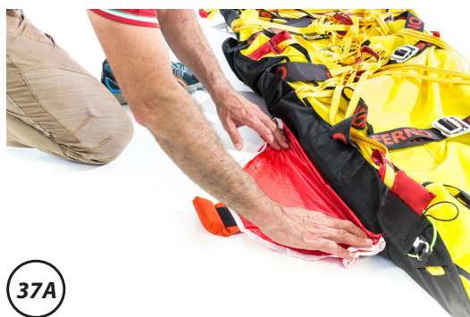
Figure 37 – Completing the insertion of the sail in its pocket
