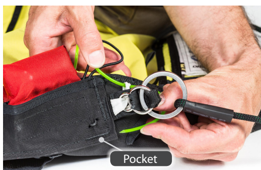
Figure 47 – Replacing the green string in the pocket
