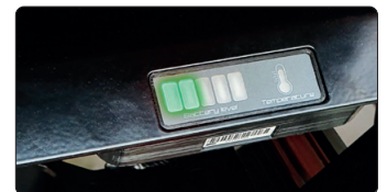
Battery capacity indicator provides real-time feedback. Temperature alert indicator warns of low battery temperature or when an electronic component becomes too hot
