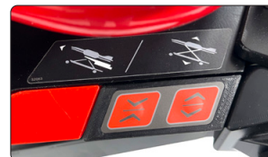
Intuitive control panel buttons for raising and lowering stretcher legs
