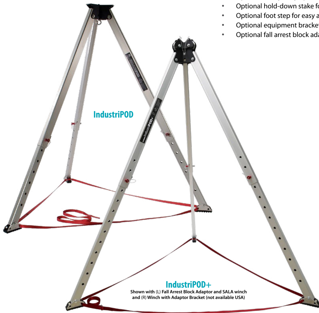
The advanced IndustriPOD+ has a one-piece fabricated steel head with two integrated 70mm sheave pulleys and three 360kg stabilisation anchor points
